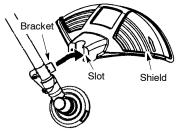
3. Secure shield to bracket with bolt.
